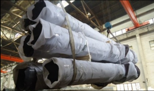
Poles are bundled together prior to being loaded into the container. When rollers are used, they are fastened to the bottom of the bundle at the end furthest from the door.
